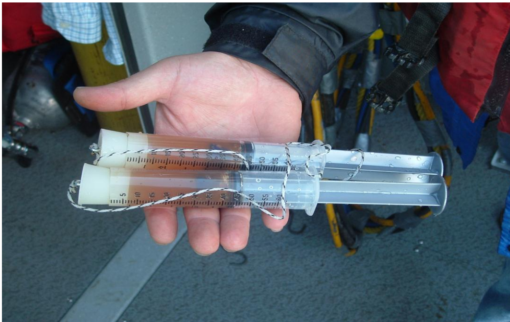
Photo 6. Corrosion Product Samples Collected for MIC Analysis
