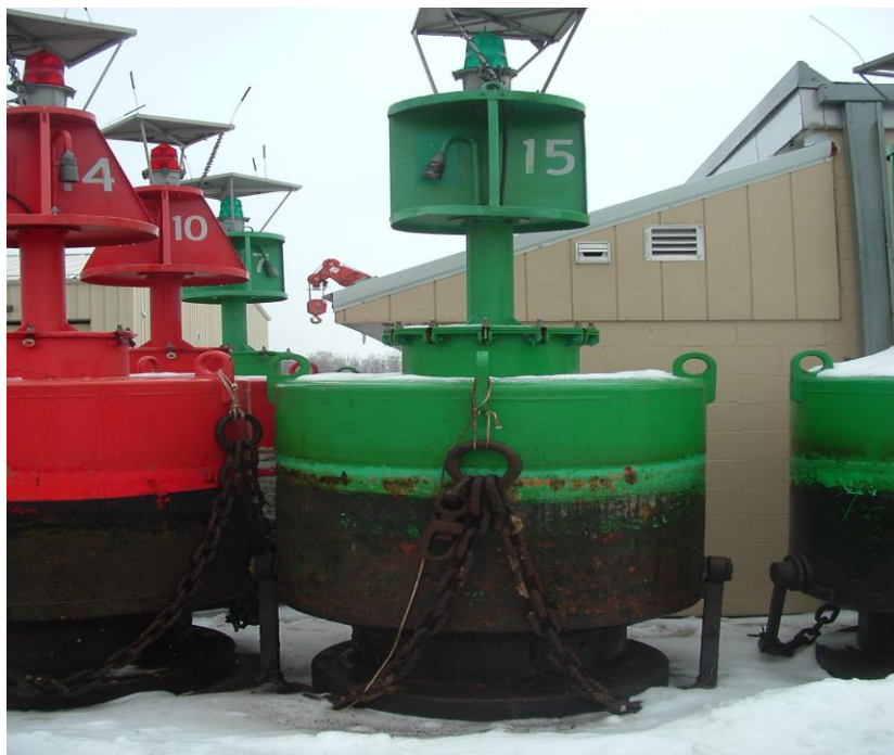
Photo 4. U.S. Coast Guard Channel Marker Buoy & Anchor Chain Bridle
